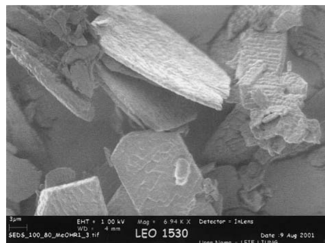
Fig. 9. Scanning electron microscopy picture of solution enhanced dispersion by supercritical fluids technique crystallized flunisolide anhydrous at 100/80 MeOH (Form IV).
